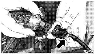
**Disconnecting Turn Signal Connector**
